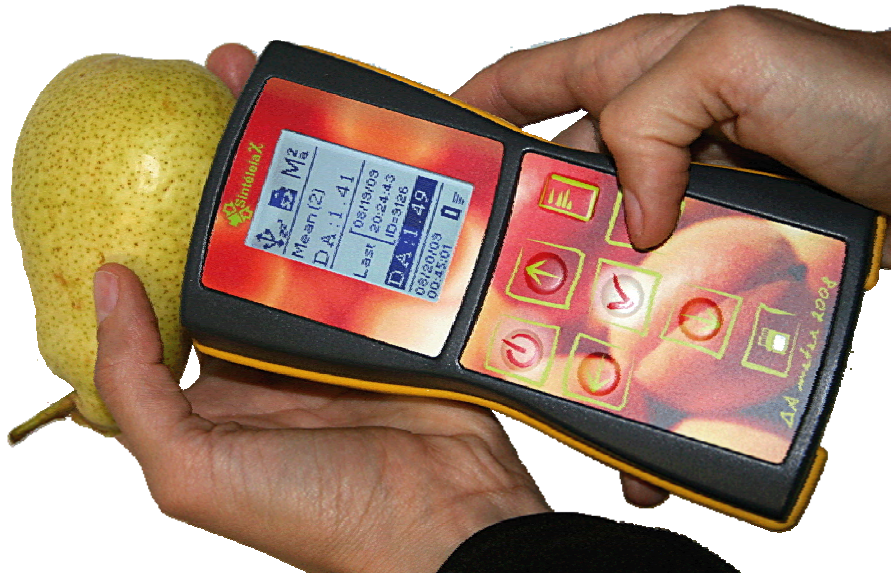
Figure 1: The DA Meter being used to take the reading of a Bon Chretien pear
