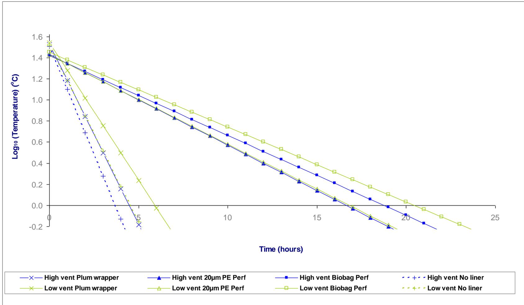
**Figure 4:** Log<sub>10</sub> fruit pulp temperature of Sapphire plums during forced-air cooling in high vent and low vent transport packaging with and without different inner packaging liners (Perf = Perforated; Non Perf = Non Perforated)
