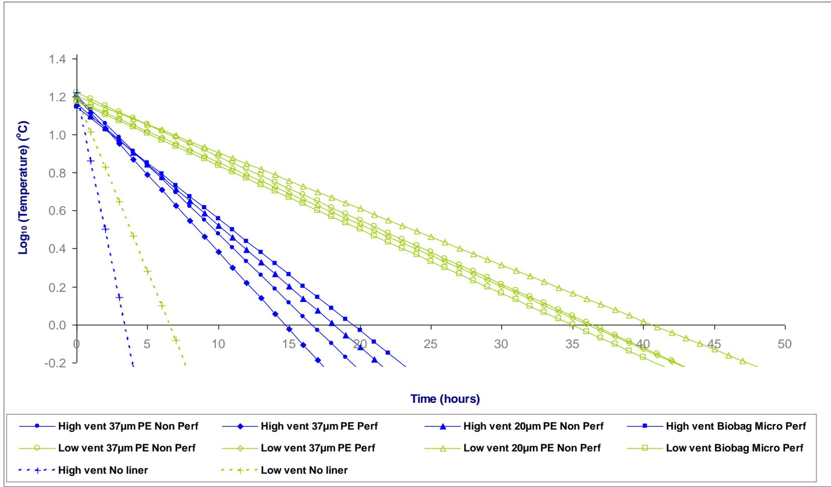
**Figure 3:** Log<sub>10</sub> fruit pulp temperature of Bon Chretien pears during forced-air cooling in high vent and low vent transport packaging with and without different inner packaging liners (Perf = Perforated; Non Perf = Non Perforated)
