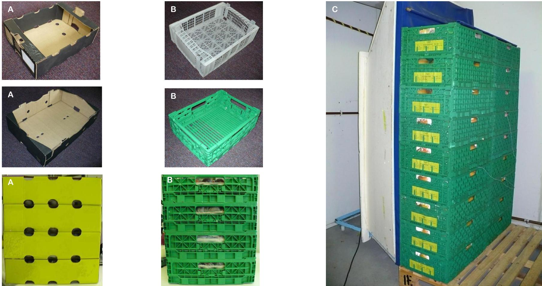
**Figure 2:** Transport packaging used for testing the effect of low vent (A) and high vent (B) packaging during forced – air cooling in an experimental stack (C) and simulated sea-freight storage of apples, pears and plums
